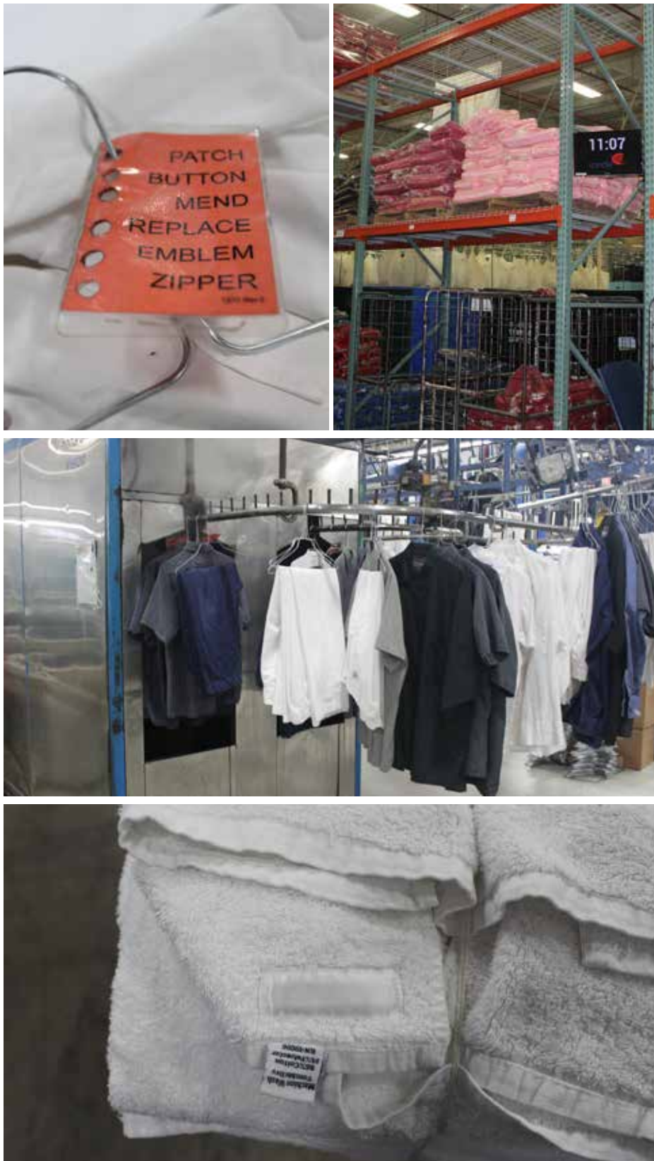
ABOVE: (clockwise from top/right) Employees place these tags on hangers using the correct hole to identify any of six common repairs that are required; a textile storage area in the plant; garments on hangers are processed in a tunnel finisher (at left); the towel at left is fitted with a sewn-in radio frequency identification tag. Miller's Textiles is in the process of placing RF tags in all its flatwork items.
