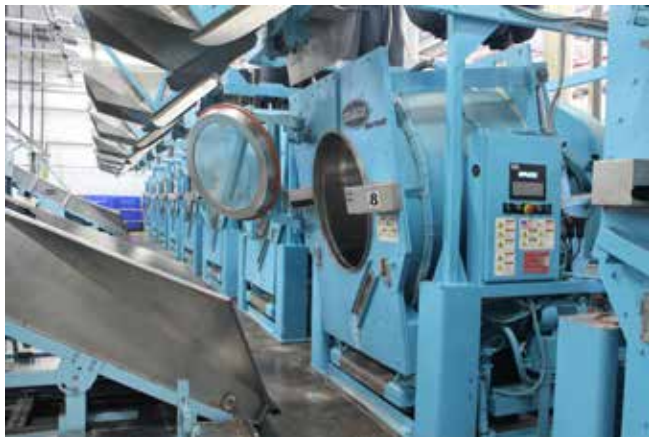
ABOVE: (clockwise, from top/left) An employee prepares to move a cart loaded with textile items fitted with radio frequency identification chips through a portal scanner. This system automatically counts and tracks the items; a view of the plant's chemical injection system; here's a line of washer/extractors and conveyors.
